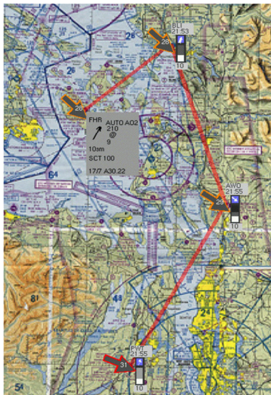
Fig. 4 Route-specific current conditions and winds aloft shown alongside a pilot-selected route. Wind velocity at the pilot selected altitude is depicted graphically with a black arrow. The airport conditions are shown using the symbolic representation (the vertical rectangle) and the textual representation. The symbolic representation shows, top to bottom, surface wind velocity, cloud coverage at altitudes from 12,000 feet down to the surface, and surface visibility. The textual representation shows all the elements available in computer briefing reports except for remarks.
